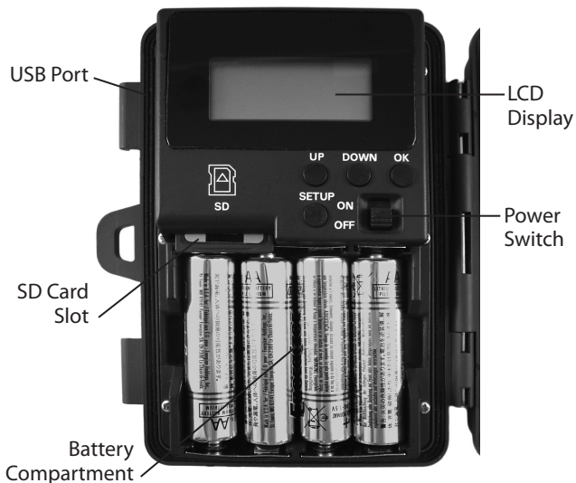
Control Panel (Front Opened)
